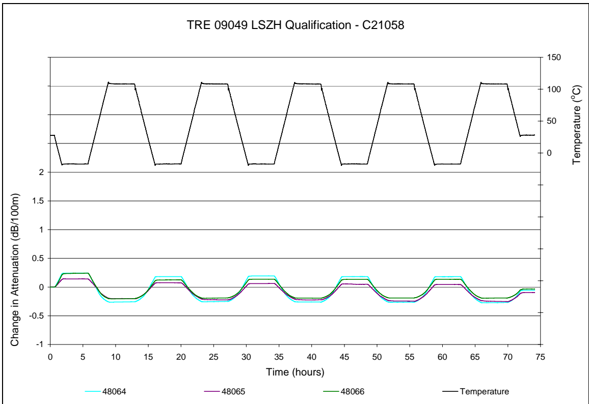
Figure 4.1c: Thermal Cycle Graph – C21058
